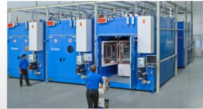
Test equipment for module and pack
